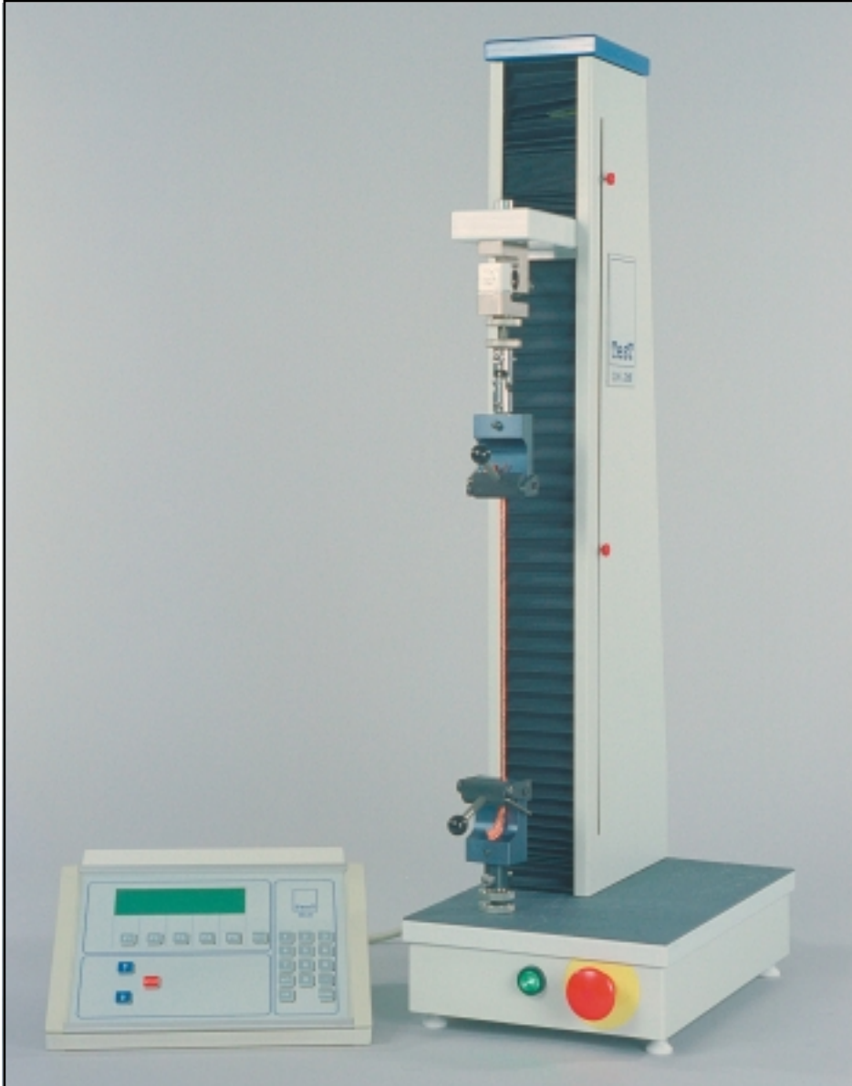
Model 106.I universal testing machine
