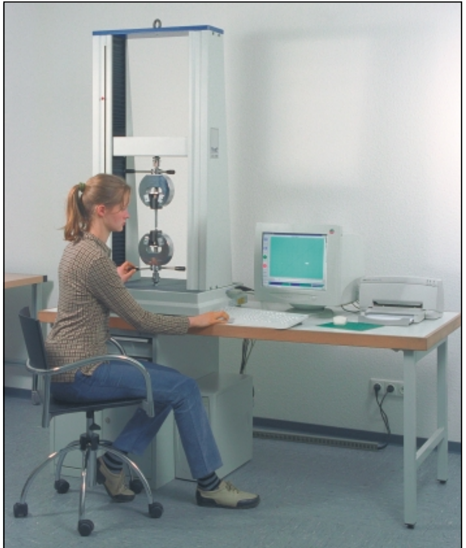
Model 112.H universal testing machine
