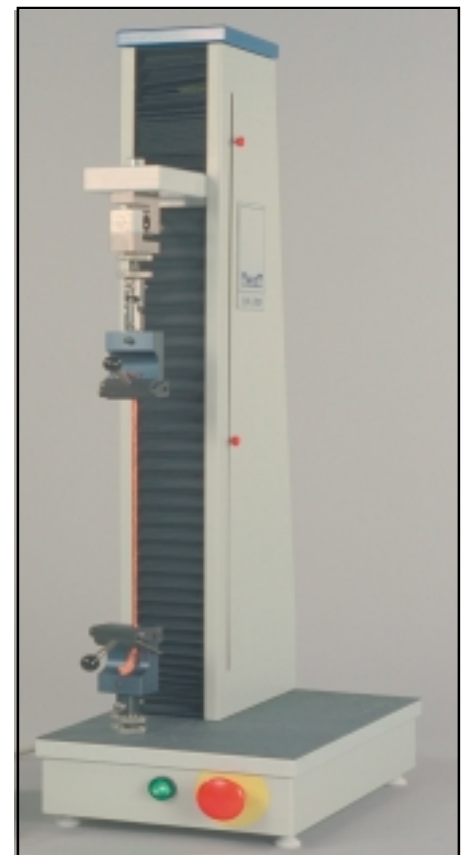
Model 106.H universal testing machine
